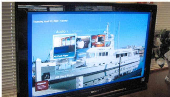
Stateroom has a mounted 42" LCD TV connected to an Xbox 360 Media Center Extender controlled by an RTI remote.
